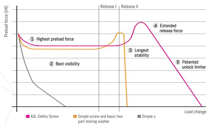
The diagram above describes the self-loosening behavior of secured and unsecured threaded fasteners under transverse loading conditions by vibration testing as per DIN 65 151.
